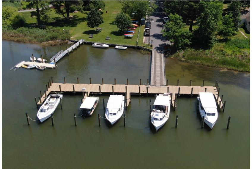
DBF provided construction documents for the realigning of the boat slips, a dredging plan and provided sufficient lengths and widths of boats that are currently using the facility.
